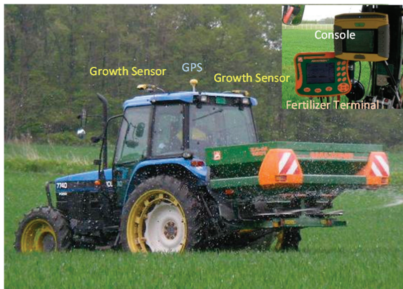
Figure 4. Components of the variable additional N application system for wheat.
