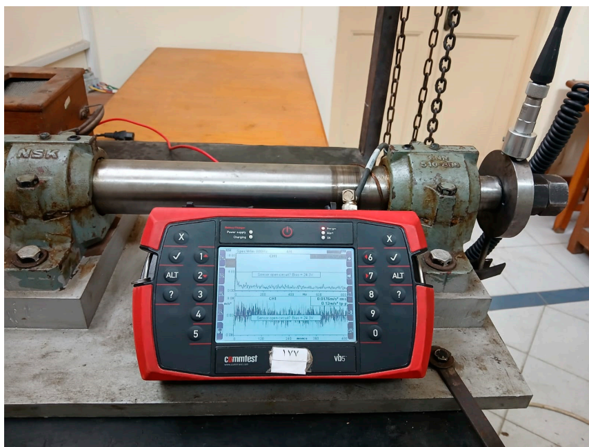
Figure 5. Vibration analysis using commtest VB5 data collector and accelerometer mounted in radial direction to the test bearings.
