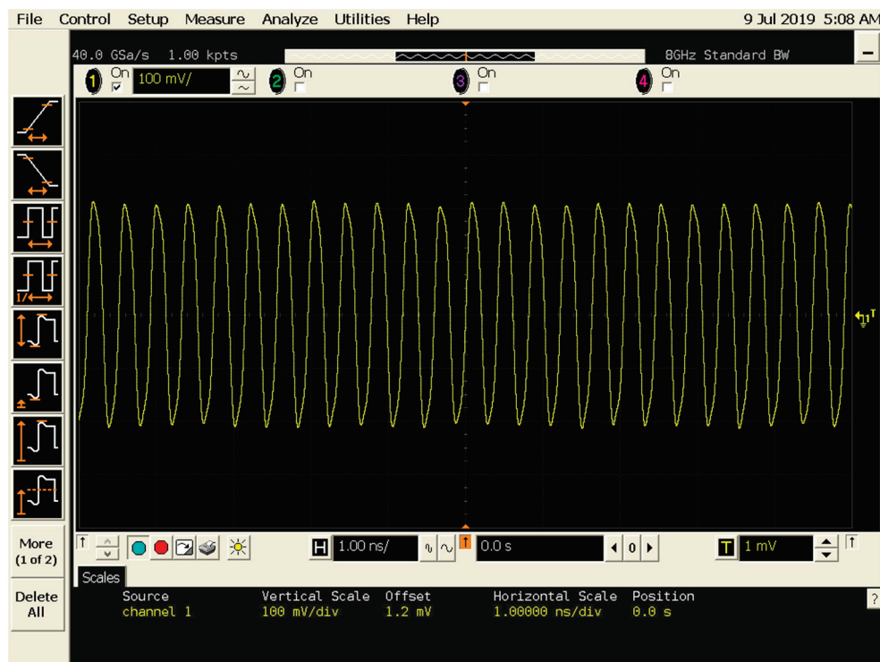
Figure 14. A time-domain screen-capture of an oscilloscope connected to the TX1 port of the AD-FMCOMMD-2/3, when the REWIRE configures the DSP_DDS.bin partial bitstream.
