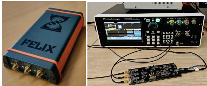
Figure 14. Picture of the FELIX board (left) hosting the Artix-7 100T for the 3-channel TDC IP-Core and the setup (right).
