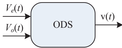
Figure 12. ODS with two inputs, P = 2 (torque, V_e(t) , and inclination angle V_o(t) ), and one output, H = 1 (vehicle speed in a longitudinal direction, v(t) ).
