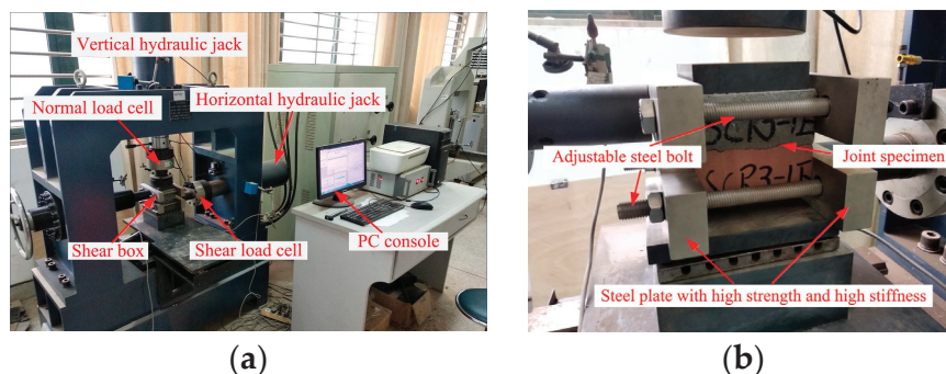
Figure 5. YZW50 electro-hydraulic servo shear test system. (a) Overall view of the apparatus; (b) the local view of shear box.
