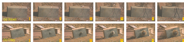
Figure 4. Rock fracture process of intact control specimen and clay-containing specimen under blast loading.
