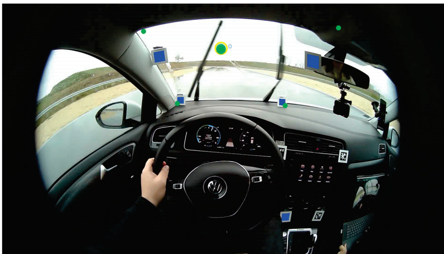
Figure 5. Gaze position (yellow circle with green fill), detected tags (blue squares), compensated tag positions (dots in the corners) and “gaze-on-road” indication (dots are green not red).
