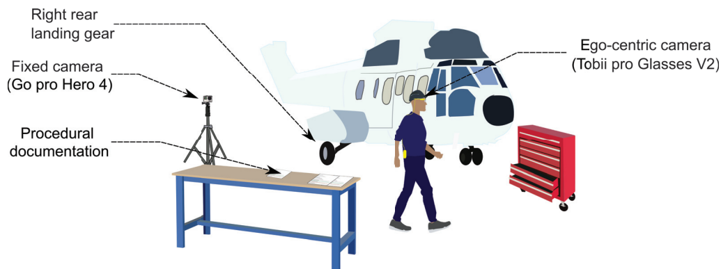
Figure 1. Aircraft maintenance activity analysis setup.
