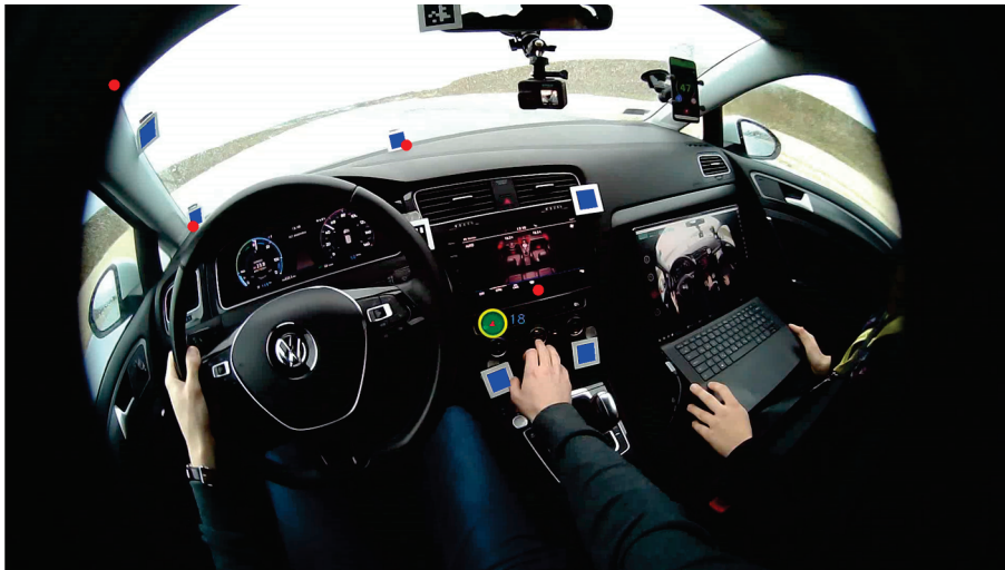
Figure 6. Gaze position (yellow circle with green fill), detected tags (blue squares), compensated tag positions (dots in the corners) and “gaze-on-road” indication (dots are red not green).
