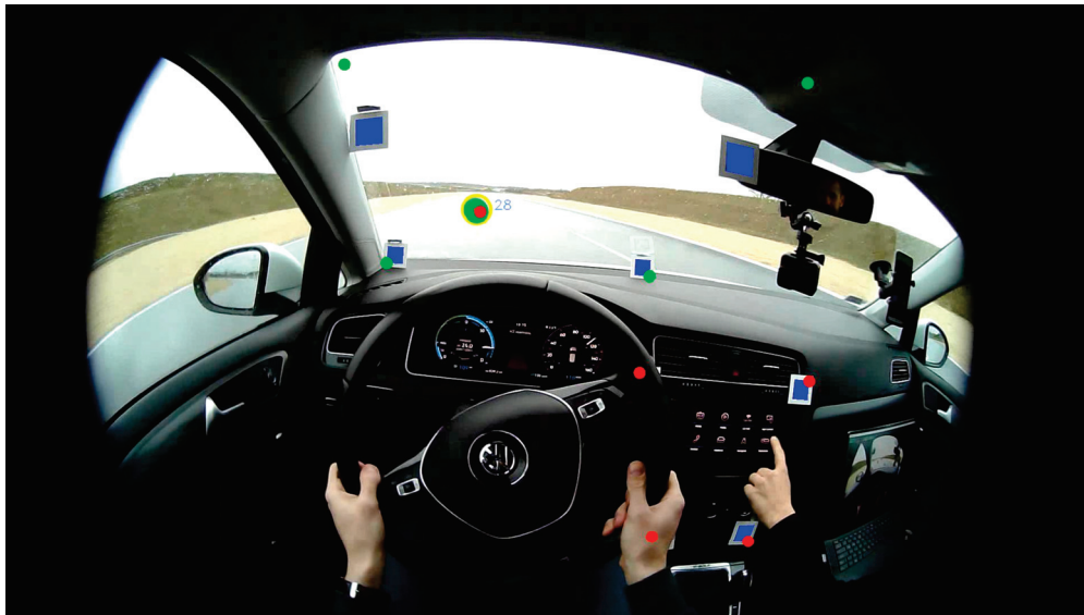
Figure 7. Incorrect recognition of the dashboard area-gaze position (yellow circle with green fill), detected tags (blue squares), compensated tag positions (dots in the corners) and “gaze on dashboard” indication (red dots).
