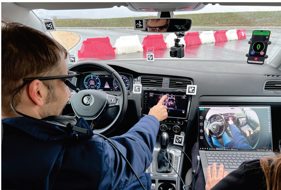
Figure 1. Test apparatus: Pupil Core eye-tracking device installed on the head of driver; ID tags in the view of driver (around windscreen and center console).
