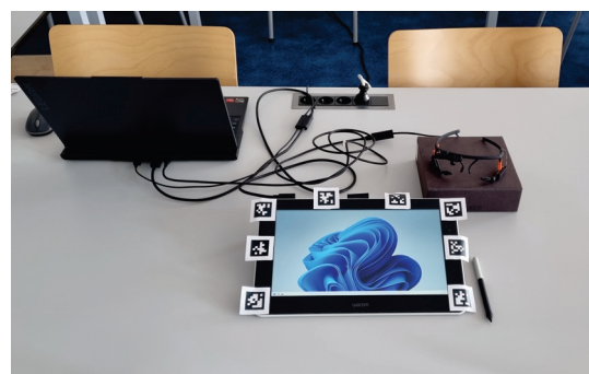
Figure 1. Stand for attention trajectory acquisition with Pupil Invisible (a) and Pupil Core (b).
