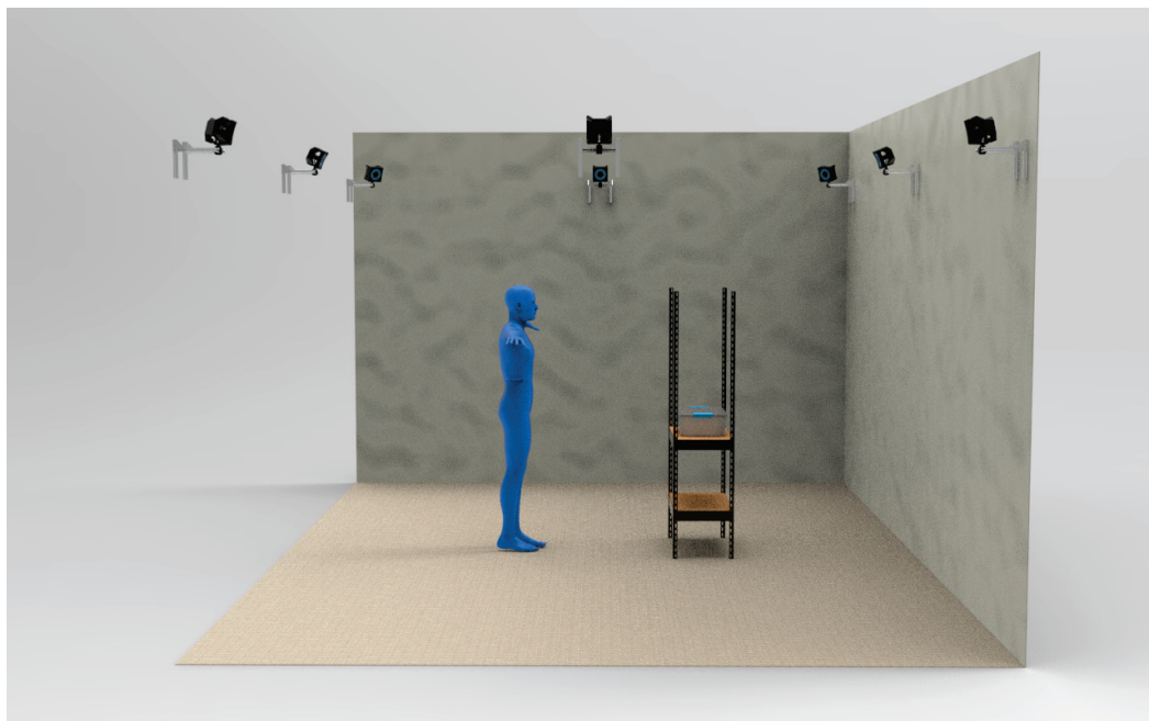
Figure 4. The motion analysis laboratory setup featuring an optoelectronic system alongside evaluation elements. The calibration volume dimensions were 5 m in length, 3 m in width, and 2 m in height.
