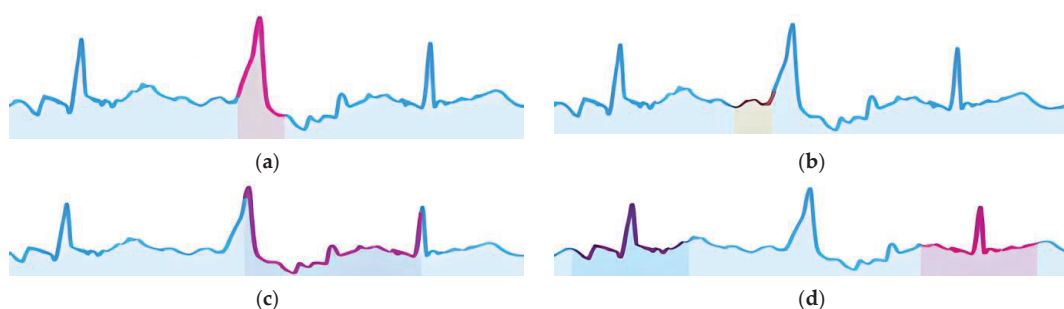
Figure 22. Visual confirmation of feature “Fusion of Ventricular Extrasystole” in an ECG, illustrating (a) an extended and deformed QRS complex highlighted in pink to indicate abnormal morphology, (b) the absence of the P peak marked in light brown to show missing atrial depolarization, (c) the lack of a compensatory pause emphasized with magenta to highlight the abnormal rhythm recovery, and (d) ventricular extrasystole highlighted in purple and pink that occurs between normal cardiac cycles.
