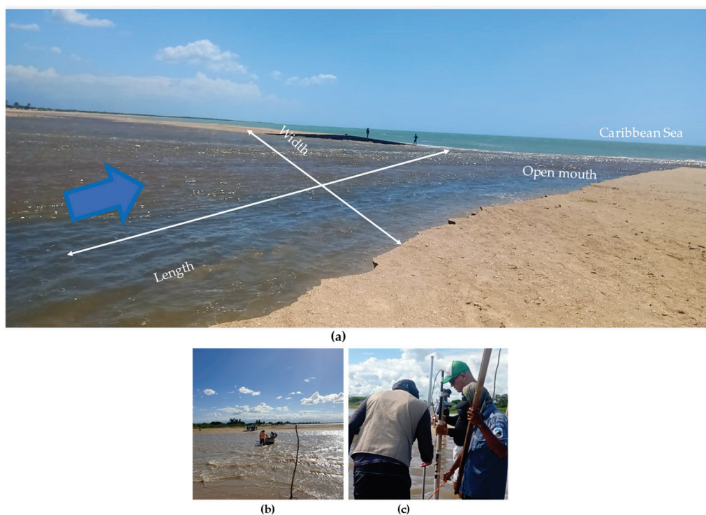
Figure 21. Details of the mouth and velocity measurements: (a) lagoon during an “open period”; (b) Our vehicle for surveying the cross-section; (c) Manual measurement of depth and velocity.
