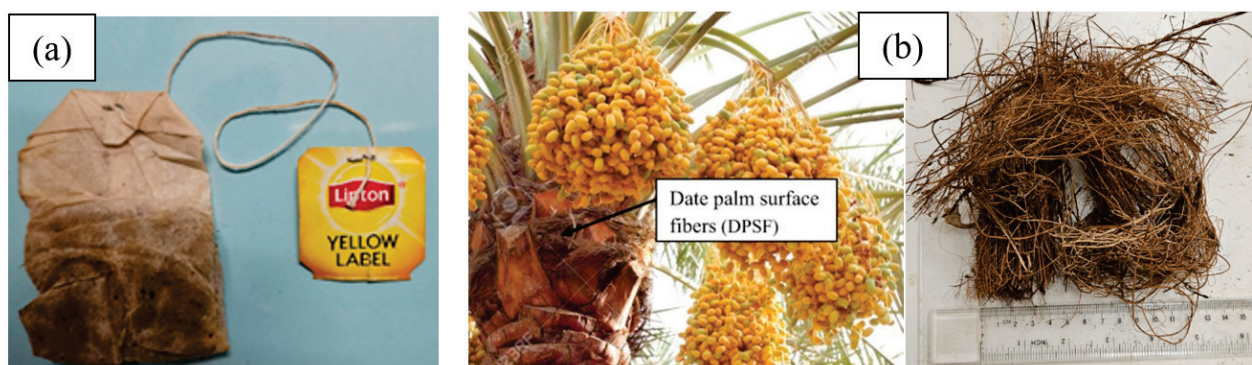
Figure 1. Raw wasted materials; (a) details of a tea bag showing the string, bag, label, and two staple pins, and (b) date palm surface fibers and their cut pieces.
