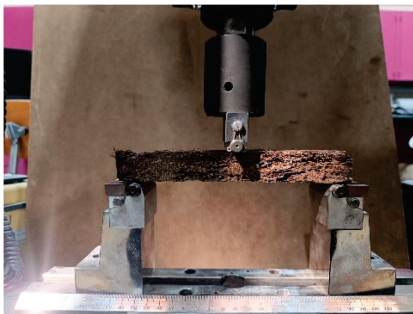
Figure 7. The universal testing machine (UTM, INSTRON 5984) used for the bending test.
