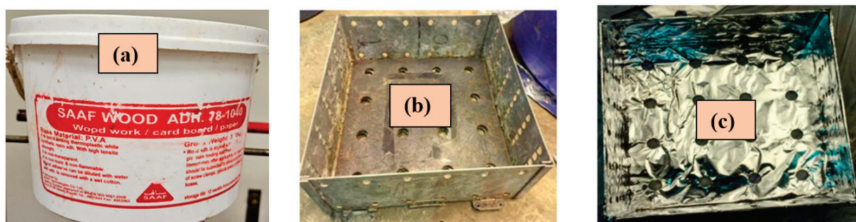
Figure 3. Resin and the stainless steel mold; (a) bucket of polyvinyl acetate (PVA) resin (wood adhesive), (b) the mold before covering with aluminum foil sheets, (c) after covering.
