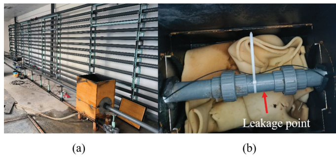
Figure 5. (a) Simulating water pipeline; (b) leakage point.
