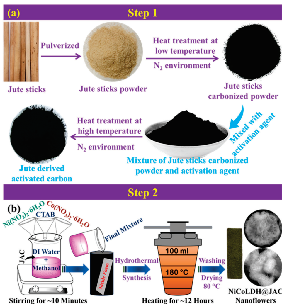
Figure 5. (a) Illustration of the JAC fabrication process involving a two-step pyrolysis method, and (b) detailed schematic of the in situ synthesis approach for growing NiCoLDH@JAC nanoflower structures. Reproduced with permission [89].
