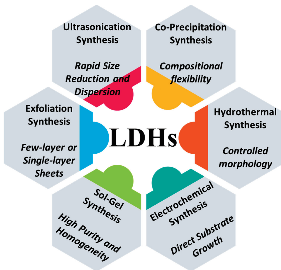
Figure 13. Schematic illustration of the advantages associated with different synthesis methods for LDHs.
