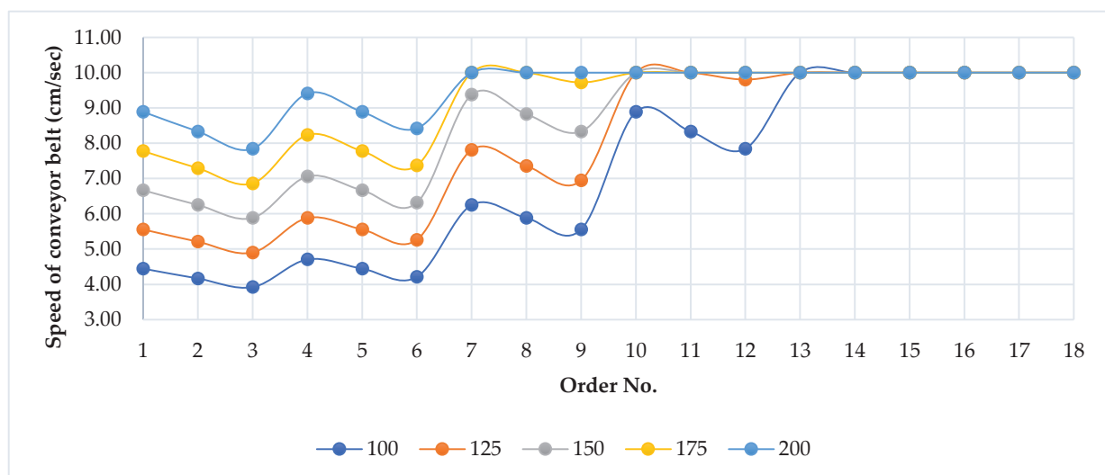
Figure 6. The impact of the yogurt nozzle's feed rate on the speed of the conveyor belt when upper limit of the speed (10 cm/s) is considered.
