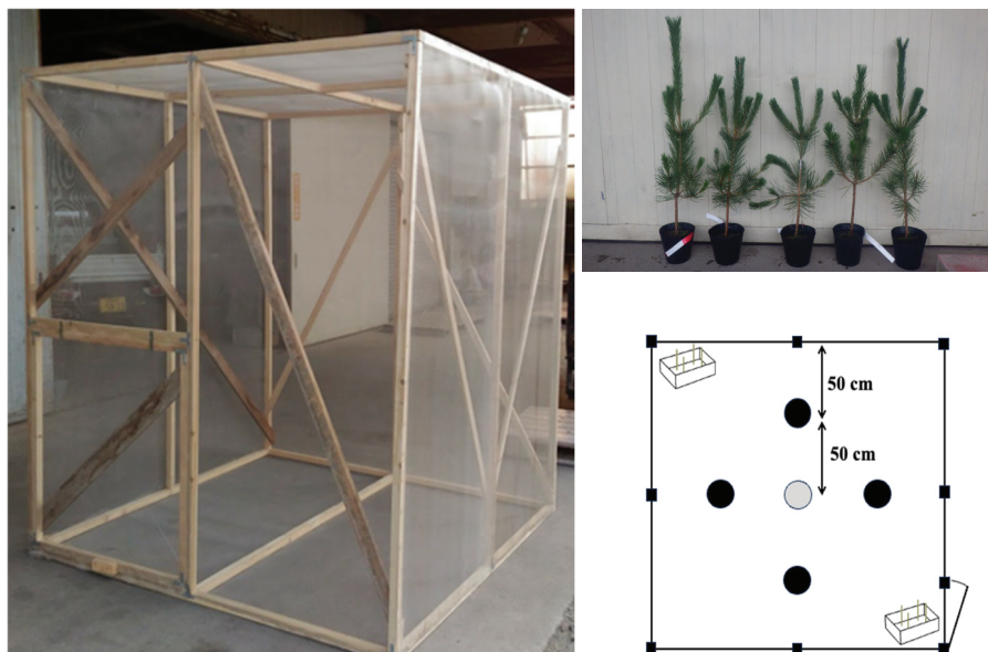
Figure 2. Mesh cage used for the Monochamus beetle release experiments (left). Five potted pine seedlings were used in each experiment: the seedling placed at the center was an artificially latently infected tree inoculated with nematodes (top right). The arrangement of the seedlings within the cage is shown in the schematic diagram (bottom right). An artificially made latent carrier seedling was pre-inoculated with 5000 Bx nematodes, and its cessation of resin exudation was confirmed 2 days prior to each experiment, then placed in the center. Insect release boxes were placed in two corners of the cage. In each, three male or three female sawyer beetles were placed. (Modified and reproduced from Ishiguro and Futai [13]).
