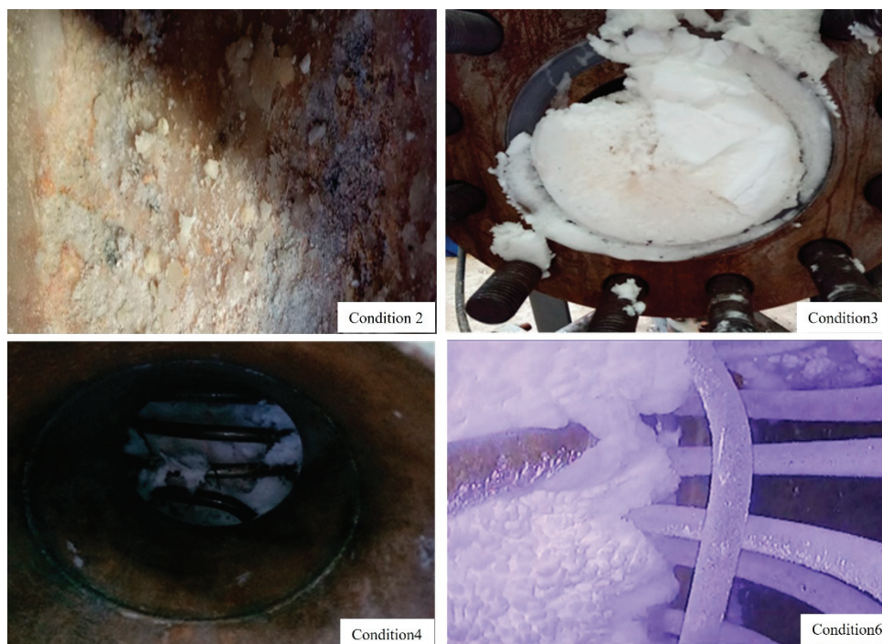
Figure 6. The synthetic products and their distribution and state in the reactor.
