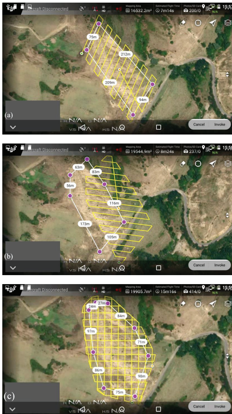
Figure 2. UAS trajectories of data acquisition designed by DJI GS RTK app for Android, version: v. 2.2.5-GSP: (a) nadir—single strip with gimbal pitch angle at 90°; (b) oblique—single strip with gimbal pitch angle at 45°; (c) oblique—cross strip with gimbal pitch angle at 60°.
