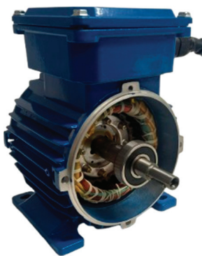
Figure 1. Three-phase squirrel-cage motor used as the prototype's base, with the side cover removed.
