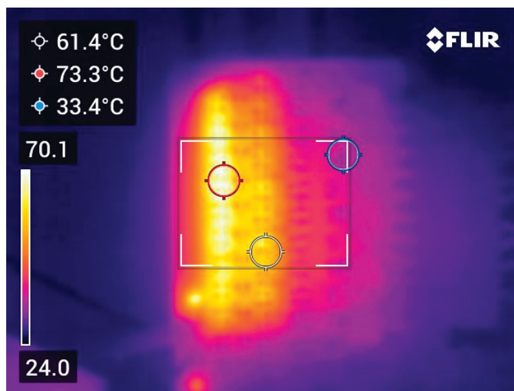
Figure 24. Full-scale BMS prototype experimental results: Temperature of the switched inductor circuit components during a long-time balancing operation.
