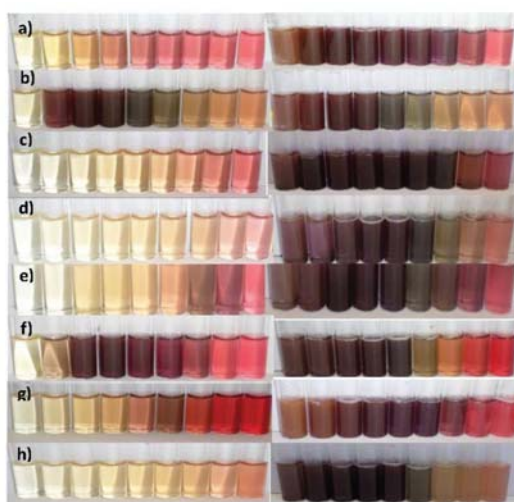
Figure 1. Response of mixtures of \text{Au}^{3+} salt and musts obtained from (a) Cabernet; (b) Garnacha; (c) Juan García; (d) Mencía Secano; (e) Mencía Regadío; (f) Prieto Picudo; (g) Rufete and (h) Tempranillo grapes. Left column corresponds to photographs taken 5 min after the mixture. Right column corresponds to photographs taken 3 h after the mixture. Ten tubes inside each picture correspond to increasing \text{Au}^{3+} :must ratios as indicated in Table 1.
