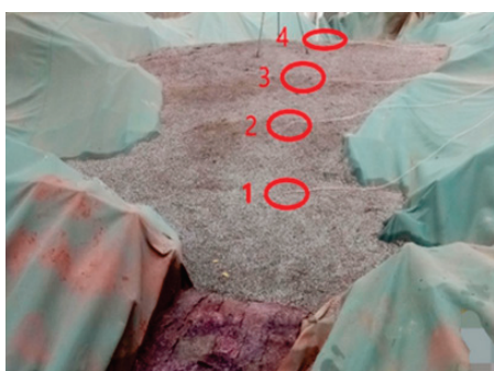
Figure 8. Buried pore water pressure gauges.
