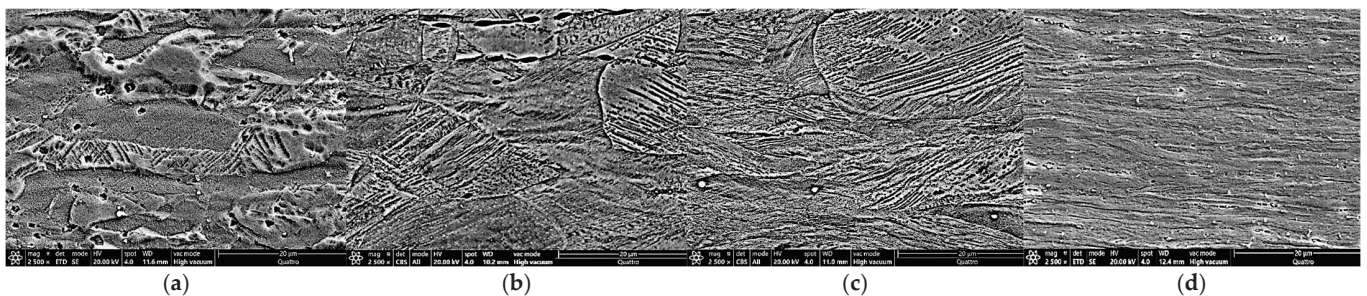
Figure 12. Microstructure of samples deformed at 0 °C: (a) 10% deformation, (b) 30% deformation, (c) 50% deformation, (d) 70% deformation.
