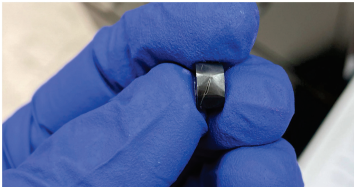
Figure 1. Handheld B_{4+\delta}C sample synthesized by the spark plasma sintering process. The image shown is during the polishing process, and the silver-colored streaks are from molybdenum foil surrounding the sample that still needs to be removed.
