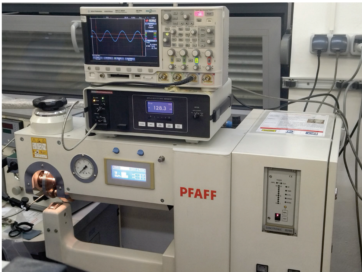
Figure 3. A measuring setup on the machine for welding polymer materials.
