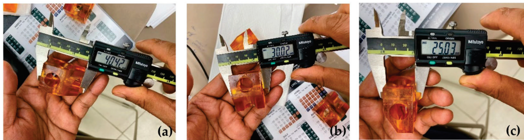
Figure 12. Three-dimensional-printed specimen made from tuned model and error measurement (a) in X, (b) in Y, and (c) in Z directions.
