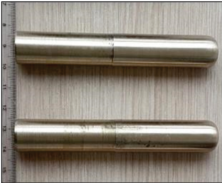
Figure 2. SAE 430B forming tools.
