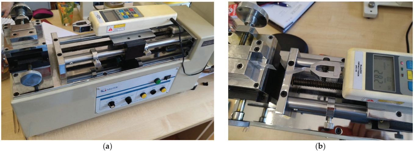
Figure 5. The measuring system for measuring breaking forces of an ultrasonic welded joint (a), test clamps with a test specimen after tearing (b).
