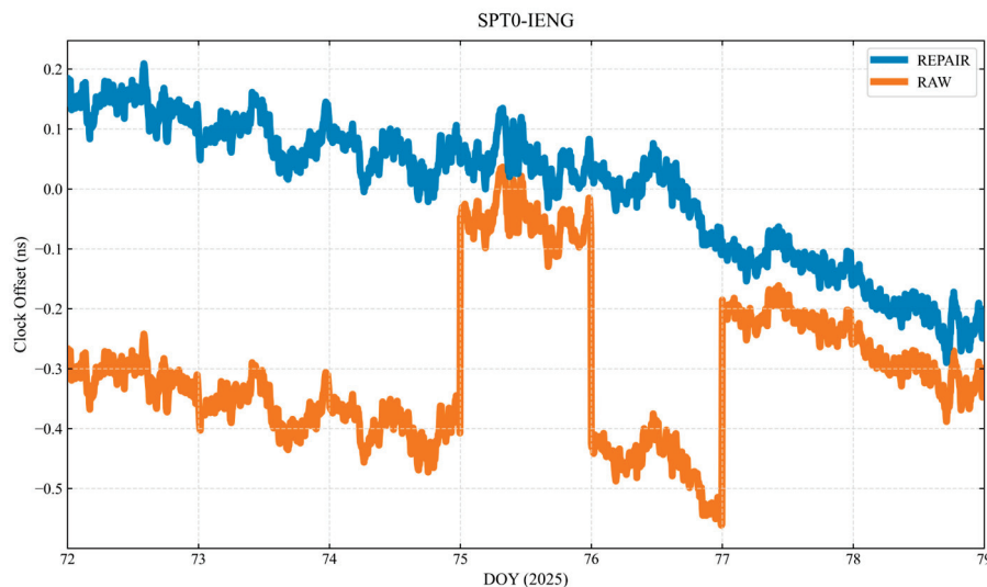
Figure 6. Comparison of day-boundary discontinuity repair for the SPT0–IENG (about 1457 km) link over 7 days. The blue curve shows the time link before repair, and the orange curve shows the result after repair.
