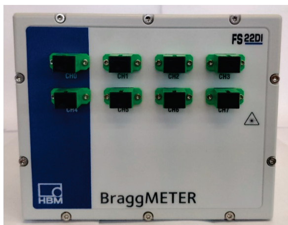
Figure 1. Optical interrogator used in the present work.
