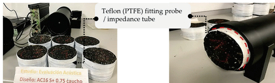
Figure 2. Impedance tube and specimens of asphalt mixtures with PTFE on their lateral surface.
