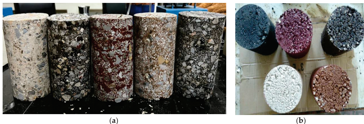
Figure 14. Dynamic modulus samples (a) after core cutting and (b) before core cutting.
