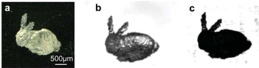
Figure 4. Comparison of silhouette images of a 3D printed bunny model using visible and UV light. (a) optical microscope image of an epoxy-based resin model of a bunny, produced using micro-stereolithography; (b) silhouette image obtained with visible transmitted light; and, (c) silhouette image obtained with UV transmitted light.
