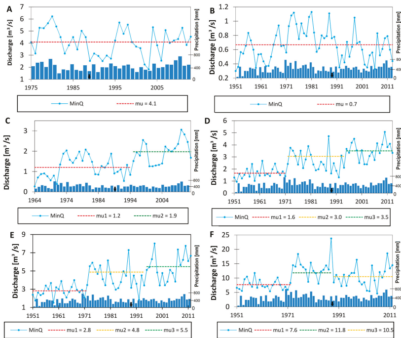
Figure 3. Annual minimum discharge for selected gauge stations of the Upper Narew Catchment: (A) Fasty, (B) Narewka, (C) Bondary, (D) Narew, (E) Suraż, and (F) Strękowa Góra. “mu” stands for the average value of each time period. The black arrow indicates the year the SR started operation.
