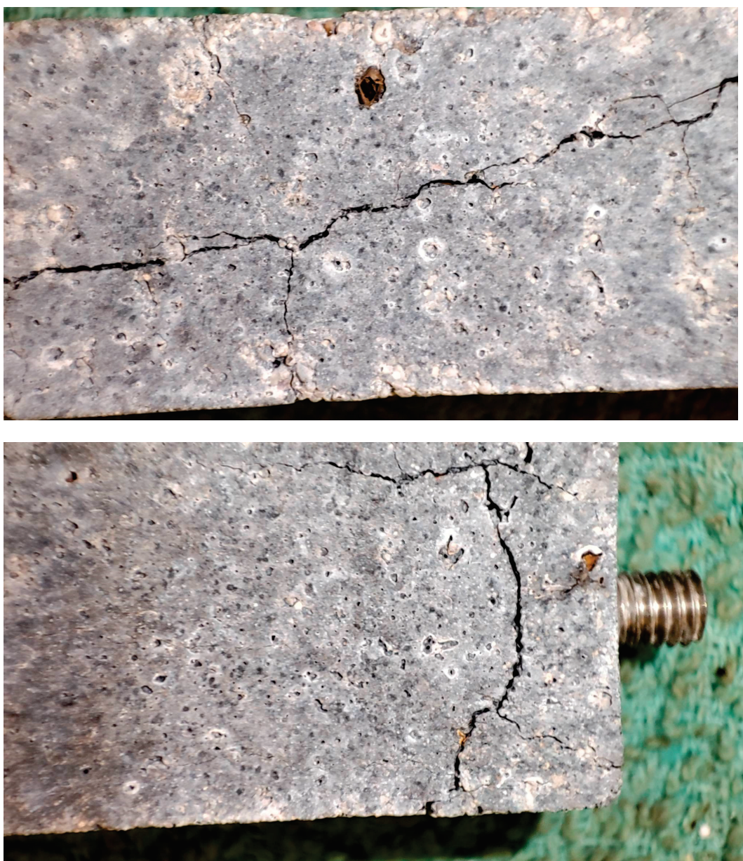
Figure 7. Cracks in samples with 20% addition of compacted microsilica.
