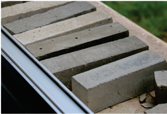
Figure 2. Carbonation depth testing made by exposing specimens in natural atmosphere.
