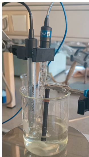
Figure 5. The setup used for electrolysis.
