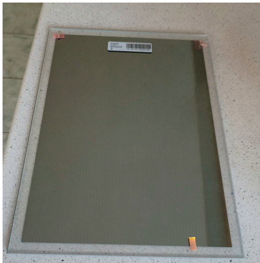
Figure 2. The CIGS photovoltaic panel from NICE Solar Energy GmbH, which was utilized for laboratory studies.
