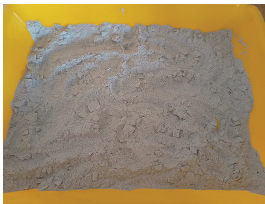
Figure 3. The ground and homogenized CIGS photovoltaic panel prepared for laboratory studies.
