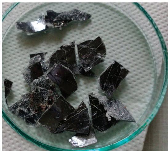
Figure 4. The absorber layer of the CIGS panel.
