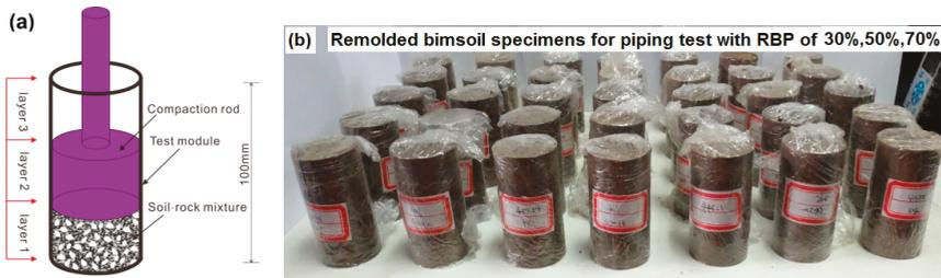
**Figure 3.** Bimsoil specimens used in the piping erosion test. (a. Compact test is used to prepare the bimsoil specimens, and the specimen was compacted with three layers; b. Partial remolded bimsoil specimens for the piping erosion test).
