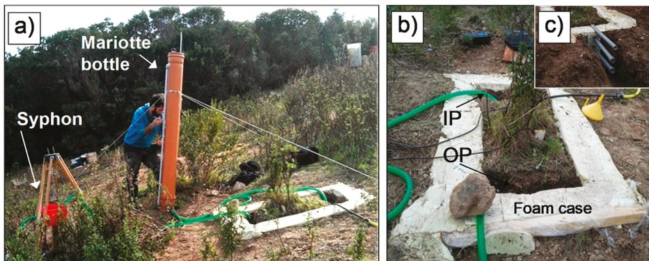
**Figure 1.** (a) Field equipment to determine lateral saturated soil hydraulic conductivities in the monoliths MA, MB and MC; (b) soil monolith encased with polyurethane foam, with signed inflow (IP) and outflow (OP) pits; (c) spillway pipes inserted in the OP foam of the monolith MD to set the water level and collect the drainage.
