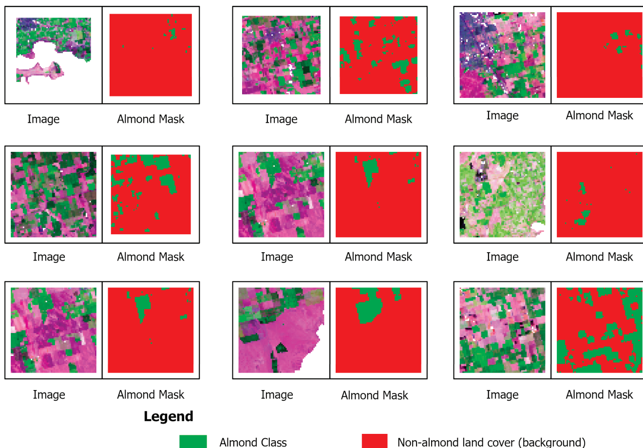
Figure 2. Sample Landsat image chips and corresponding almond masks used for model training. Each pair shows a satellite image with a 5,4,3 as R,G,B color composite which highlights vegetation as shades of green, bare soil as magenta, and urban as purple ( left ) and its binary classification mask ( right ), where green denotes almond land cover and red indicates non-almond land cover (background). The masks were derived from USDA Cropland Data Layer labels.
