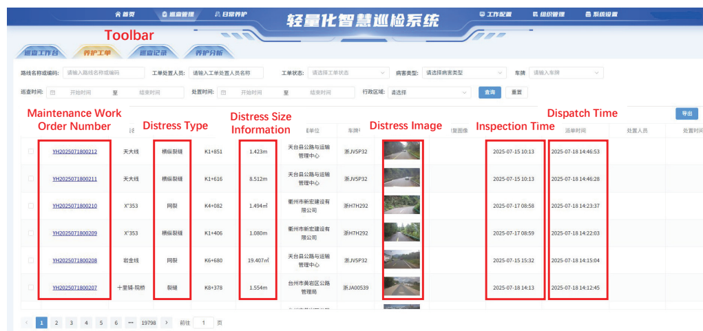
Figure 9. Maintenance work orders.
