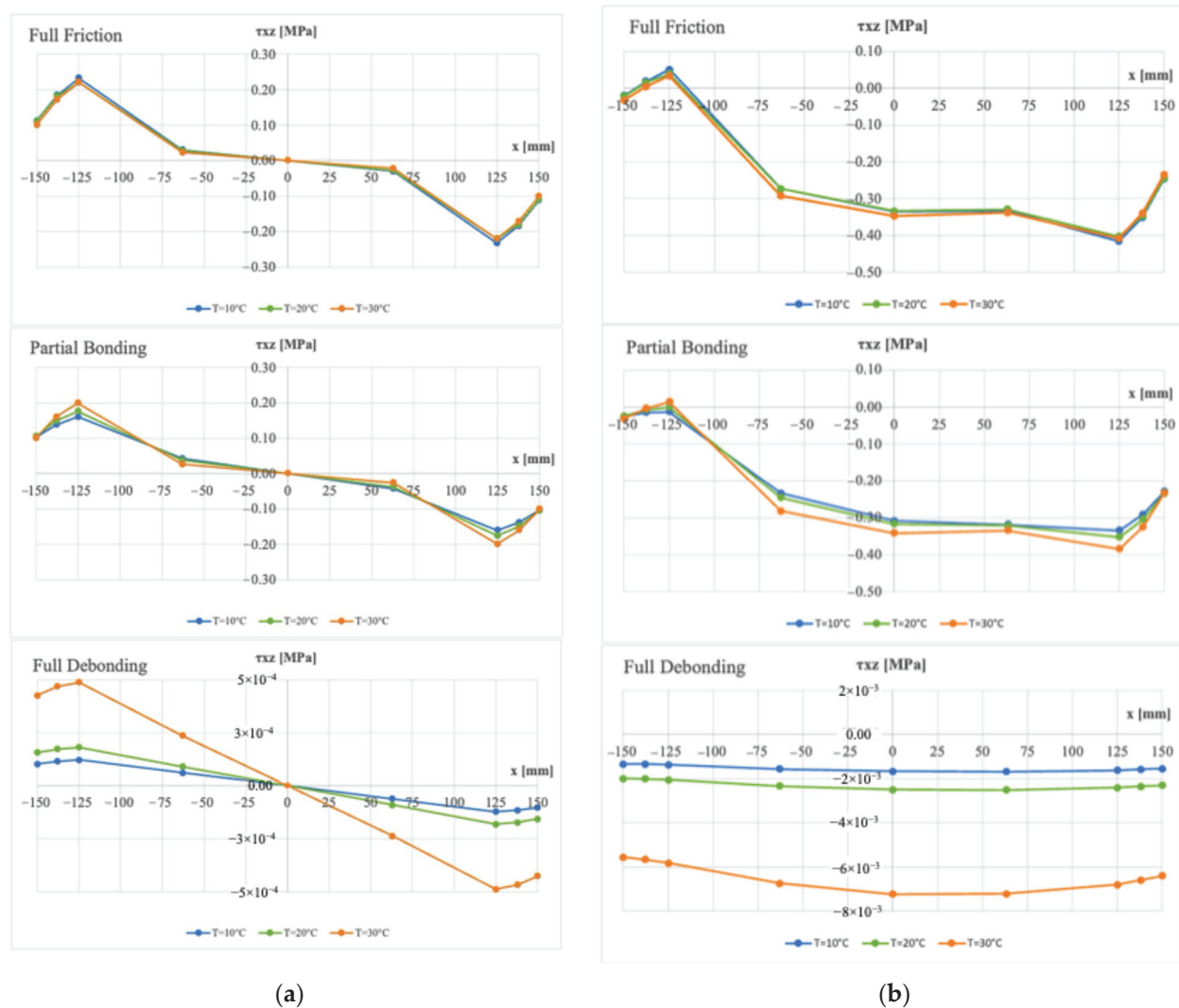
Figure 9. Shear stress trend at the wear–binder interface, under different bonding conditions and temperatures (a) for loading configuration 1; (b) for loading configuration 2.
