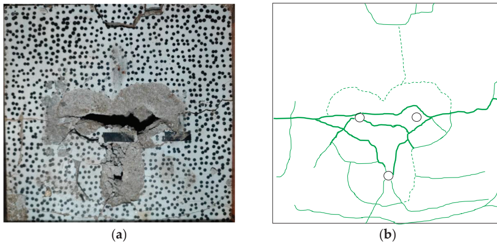
Figure 19. The blasting effect of rock plate cracking under millisecond blasting: (a) rock slab fragmentation; (b) crack extension pattern. The green lines represent only the location of the cracks.
