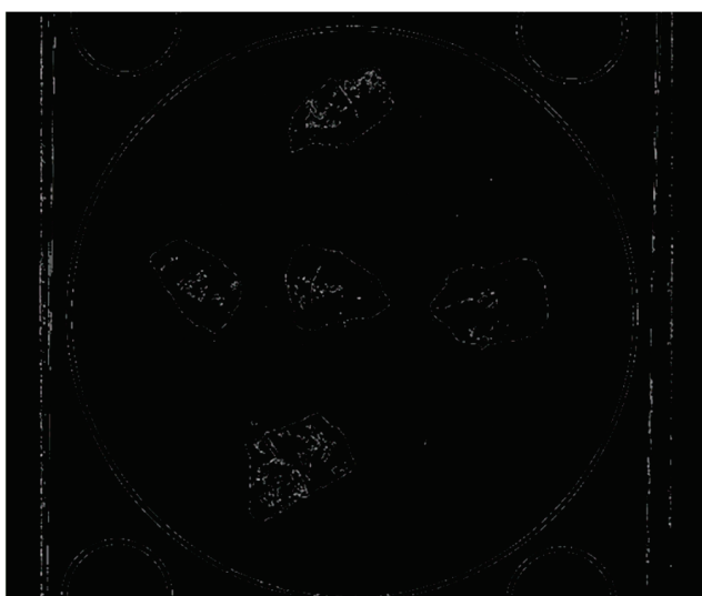
Figure 8. The contour search algorithm is used for the boundaries obtained via Canny operator.
