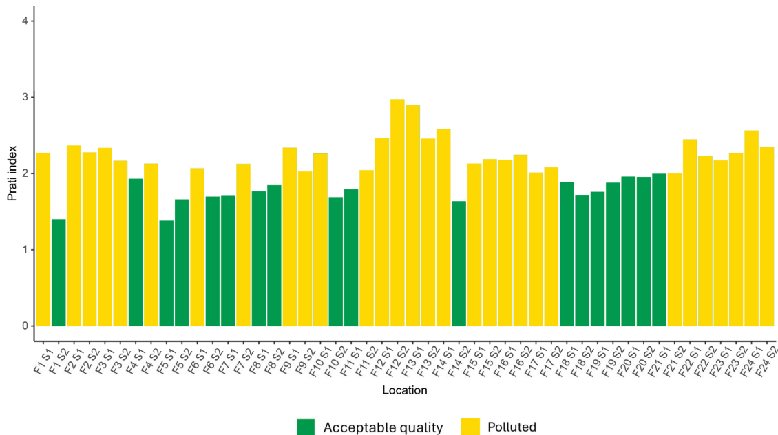
Figure 3. Spatial distribution of Prati index and water quality classification along the Lieve River. Green bars represent “Acceptable quality” (Prati index \leq 2.0 ); Yellow bars represent “Polluted” (Prati index > 2.0 ).
