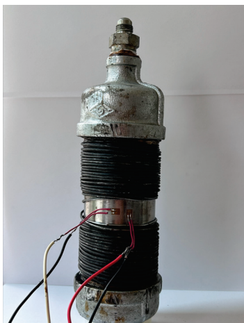
Figure 5. Prototype of a metallic-reinforced pressure vessel.
