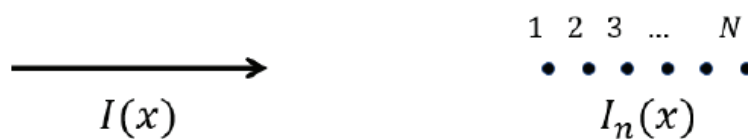
Figure 7. Schematic representation of a continuous current source (on the left) and of a discrete current source obtained by sampling the continuous source (on the right).
