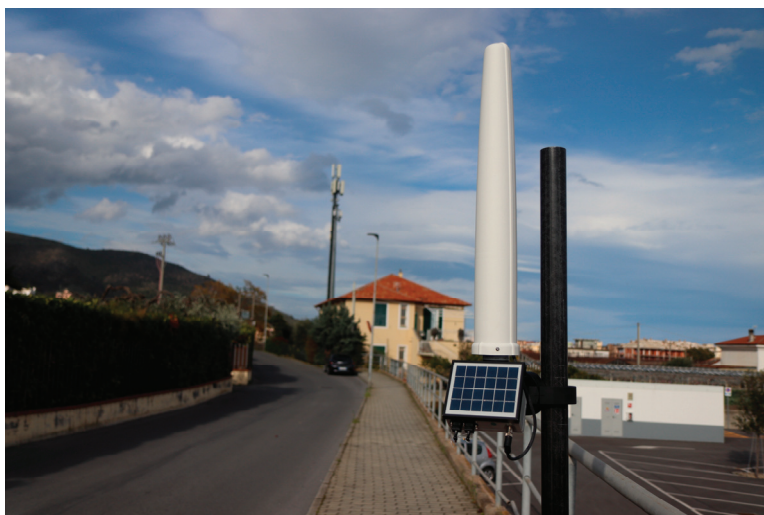
Figure 1. An example of a battery-operated EMF area monitor in a real application scenario (courtesy of NARDA Safety Test Solutions S.r.l.).
