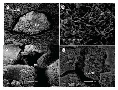
**Figure 7.** SEM images of clay minerals in undeformed sandstones. (**A**) Feldspar grain surrounded by fractured smectite. (**B**) Well developed smectite flakes inside a pore. (**C**) Pore-line illite coatings capping quartz grains. (**D**) Mixed layers of smectite and illite. Key: Sme—smectite; Fsp—feldspar; Ill—illite.
