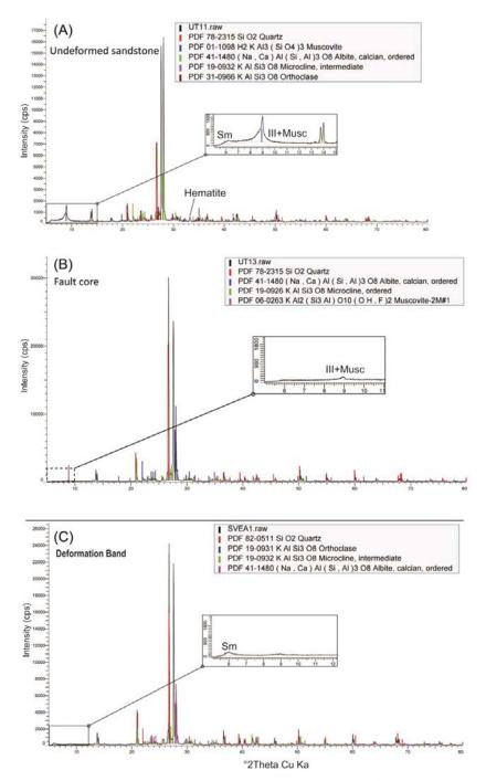
Figure 8. Examples of XRD analyses on bulk samples representative of undeformed sandstone (A), foliated cataclasite in fault core rock (B) and deformation band (C).
