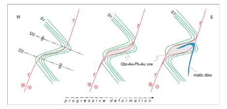
**Figure 15.** Baccu Locci/San Riccardo mine: scheme of the geometric relationships between foliation, faults, mafic dikes, and Qtz–As–Pb sulphide veins. See the location of this structure in the larger LD1 antiform in the cross-section in Figures 3 and 4.
