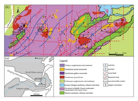
**Figure 1.** Geological map of the study area: (a) simplified tectonic map showing the location of the TOD; and (b) geological map of the TOD showing the locations of copper occurrences, modified from a 1:50,000 scale geological map [52] and [37,42,43,53].
