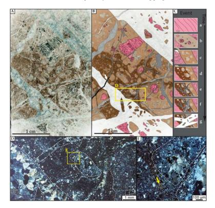
**Figure 5.** (**A**,**B**) Thin section of a polyphase cataclastic fault rock crosscut by several generations of quartz veins of the QB. White arrow indicates a late microcrystalline quartz veinlet; (**C**) simplified chronology of the events; (**D**) zoom on the different generations of clasts; and (**E**) matrix of the latest cataclastic event displaying white micas and micro-crystalline quartz.
