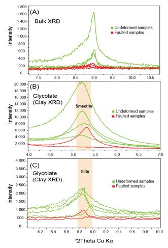
**Figure 10.** Summary diagrams showing a comparison between diffractograms of undeformed host rocks (green lines) and faulted rocks (red lines). (**A**) Bulk XRD analysis indicating that that the amount of clay minerals in the undeformed samples is higher than that in faulted samples. (**B**) The relative abundance of smectite in undeformed and faulted samples. (**C**) The relative abundance of illite in undeformed and faulted samples.
