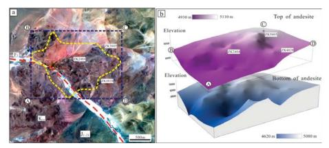
**Figure 7.** (a) High-resolution remote sensing image, and (b) a 3-D map of the Meiriqiecuo Formation andesite [31]. Red dotted lines: faults; the yellow dotted line: the boundary of the mineralized body.
