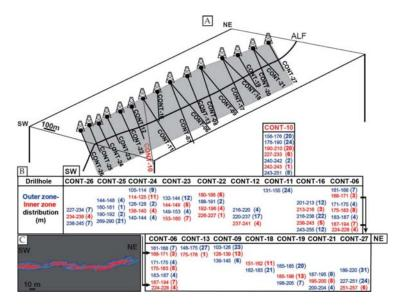
**Figure 3.** Organisation of inner (core) and outer zones of the quartz breccia (QB) crosscut in drillholes at Contact. (A) Plan view of the drill holes; (B) lateral variation in thickness of QB inner (core) and outer zones; and (C) simplified interpretative drawing of the QB intersected in drill holes (grey plane).
