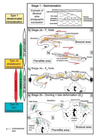
**Figure 11.** Genetic model for the formation of the three main Pb-Zn mineralization types. **Stage 1** is the disseminated Type 1 mineralization that is supposed to be syn-sedimentary. **Stage 2a** is the syn-D<sub>1</sub> Type 2a stratabound mineralization which is followed by the formation of F<sub>2</sub> folds and local remobilization of Pb-Zn mineralizations (saddle reef). **Stage 2b** represents the Type 2b late-Variscan vein mineralizations.
