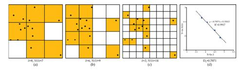
**Figure 2.** Schematic diagram of box-counting analysis: (a) 7 boxes containing target points with box size  $\delta = 8$ ; (b) 9 boxes counted with box size  $\delta = 6$ ; (c) 14 boxes counted with box size  $\delta = 3$ ; and (d) log-log plot revealing the power-law relationship of counted box number  $N(\delta)$  and box size  $\delta$ , obtaining box-counting fractal dimension  $D_B = 0.7071$ .
