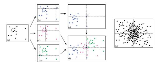
**Figure 3.** Schematic diagram for constructing a Fry plot: (**a**) the original sheet records raw points; (**b**) the origin *O* is placed on one of the raw points; (**c**) distribution pattern of raw points according to the origin *O* is transferred to the tracing sheet; (**d**,**e**) the origin *O* is re-placed on every raw point; (**f**) the tracing sheet records all distribution patterns of raw points with respect to different origins; and (**g**) Fry plot is constructed.
