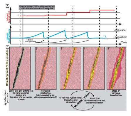
**Figure 11.** (A) Evolution of inferred fault strength (frictional shear resistance) and fluid pressure in the fault zone as a response of fluid pulse, fracturing and silica-precipitation. (**B**) Scheme depicting the succession of events that produced the QB.
