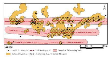
**Figure 16.** Buffer analysis showing the distribution of copper occurrences in buffered EW-trending faults and intrusions.
