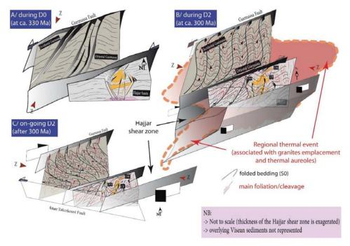
**Figure 10.** Tectono-metamorphic model of the Hajjar shear zone and associated MSD. The name of the tectonic events (D0, D2) corresponds to the tectonic events that have recently been established for the Jebilet Massif by Delchini (2018) [26]. D1 has not been identified in this study. See text for explanations.
