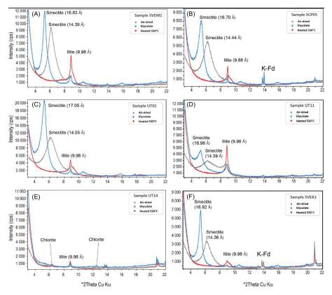
**Figure 9.** XRD diffractograms of aggregates of clay-size fractions of undeformed (**A**–**D**) and fault core (**E**) rocks, and a deformation band in a fault damage zone (**F**). Air-dried (in grey), heated at 550 °C (in red), and treated with ethylene glycol (in blue) conditions are shown.
