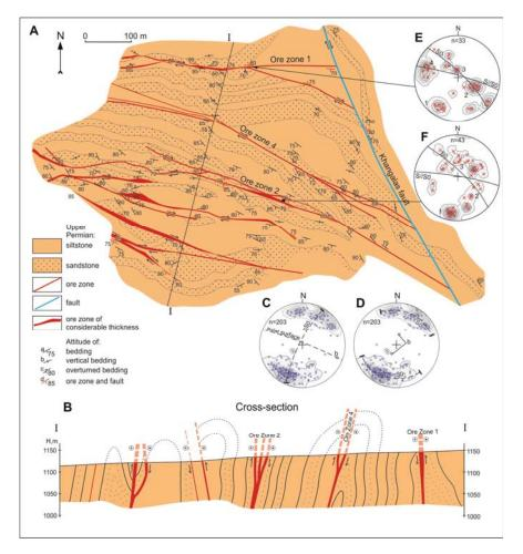
**Figure 5.** Geological sketch map and section of the Nagornoye occurrence. In (**A**), the I-I line shows the position of the cross-section (**B**). The diagrams show: (**C**,**D**) bedding poles; (**E**) quartz vein poles in Ore Zone 1; (**F**) quartz vein poles in Ore Zone 2. Contours of poles to planes (per 2% area).
