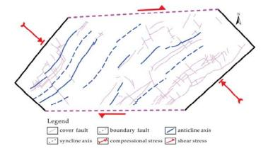
Figure 18. Stress regime during the formative process of the folds with sigmoidal axes, modified from [42].
