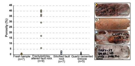
**Figure 6.** Porosity measured for fresh samples (granitic gneiss from the Contact prospect), pervasively silicified cataclastic fault rock, thick quartz veins within granitic gneiss, and clay-altered, fractured host rock (examples for each category are displayed on the right of the chart).
