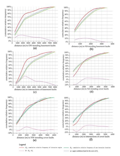
**Figure 15.** Graph of cumulative relative frequency concerning distance to (a) EW-trending faults; (b) NS-trending faults; (c) intersections of basement faults; (d) NE-trending faults; (e) NW-trending faults and (f) intersections of cover faults.
