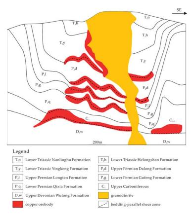
**Figure 20.** Typical cross-section of Shizishan ore field showing the characteristic stratabound skarn orebodies hosted in the folds, modified from [43].
