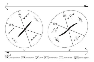
**Figure 19.** Deformation model of dextral shearing in a strike-slip fault zone, modified from [61]. (a) a structural system formed in initial stage of deformation; and (b) a rotation of structural elements during continued strike-slip shearing.
