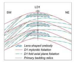
Figure 9. Schematic relationships between lens-shaped sulphide orebodies, D1 fold axial plane foliation, and D1 mylonitic foliation in the hinge zone of LD1 antiform at Spilloncargiu mine works (not to scale).
