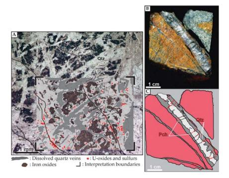
**Figure 13.** (**A**) Plane polarized light picture and interpretation drawing of a quartz vein network guiding the mineralizing fluid along its boundaries. Quartz and iron oxides display evidence for dissolution; (**B**,**C**) macroscopic drill core sample scan and interpretation drawing: Examples of a QB related quartz vein bearing pitchblende (Pch) along edges or in orthogonal microfractures.
