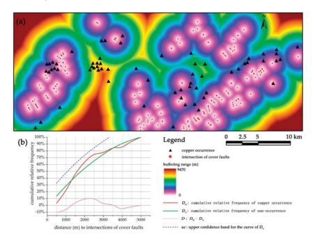
Figure 12. (a) Buffer analysis and (b) graph of cumulative relative frequency concerning distance to intersections of cover faults.
