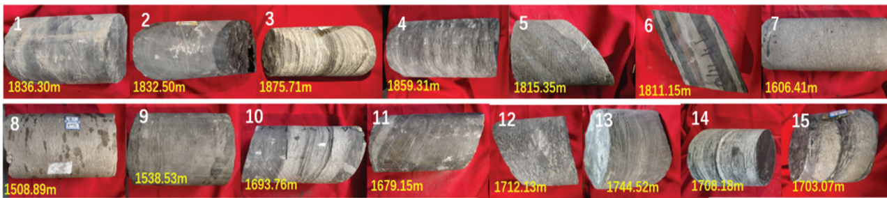
Figure 1. Core sampling during drilling at the Zhengning oilfield.
