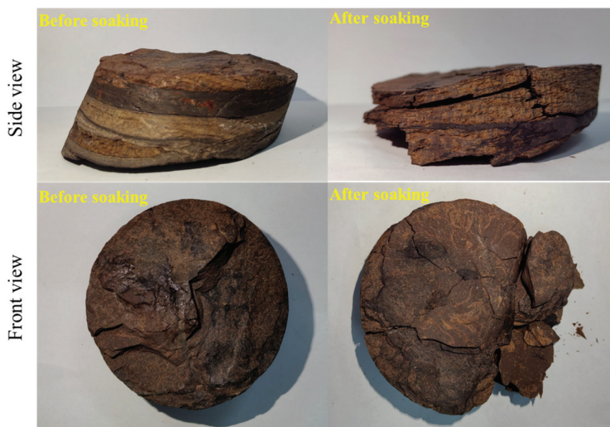
Figure 10. Comparison of main and side views of core 10 before and after soaking in distilled water.
