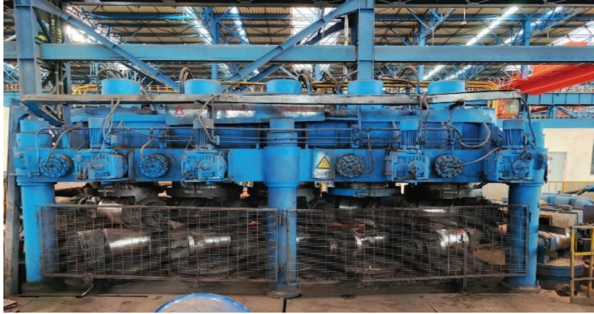
Figure 8. Eleven-roll straightening machine for bars.
