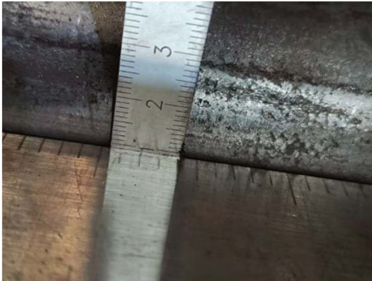
Figure 10. Straightness check after bar straightening.
