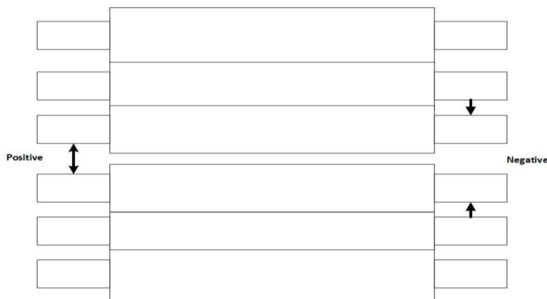
Figure 3. Asymmetric roll bending force schematic.
