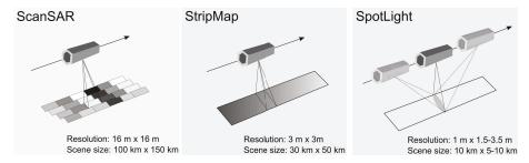
Figure 4. TerraSAR-X basic imaging modes and main configurations [62,63].
