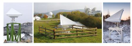
Figure 5. Corner reflectors (CRs) at geodetic observatories. CR with 0.7 m inner leg dimension at GARS O'Higgins (left), and CRs with 1.5 m inner leg dimension at Wettzell (middle) and at Metsähovi (right).
