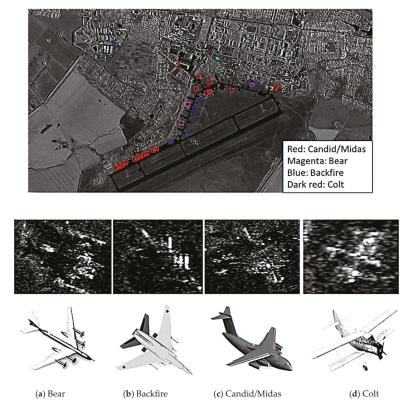
Figure 13. Target detection and classification of TerraSAR-X Staring SpotLight images for Ryazan airbase.
