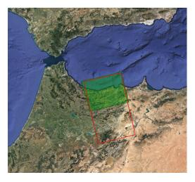
**Figure 15.** Example for scene coverage verification after data take acquisition, visualized in Google Earth. The red polygon indicates the requested scene, whereas the green polygon shows the acquired scene. In this case, a considerable part of the data take is not available, as the downlink was affected by severe weather conditions.
