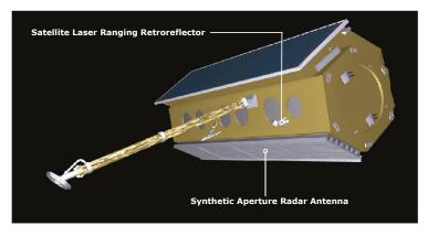
Figure 1. Illustration of TerraSAR-X with selected optical and radar payload for orbit validation.
