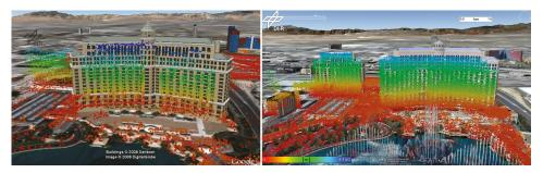
Figure 3. Comparison of the density of the 3D point cloud retrieved by PSI (left) and TomoSAR (right) of Bellagio Hotel, Las Vegas [8].
