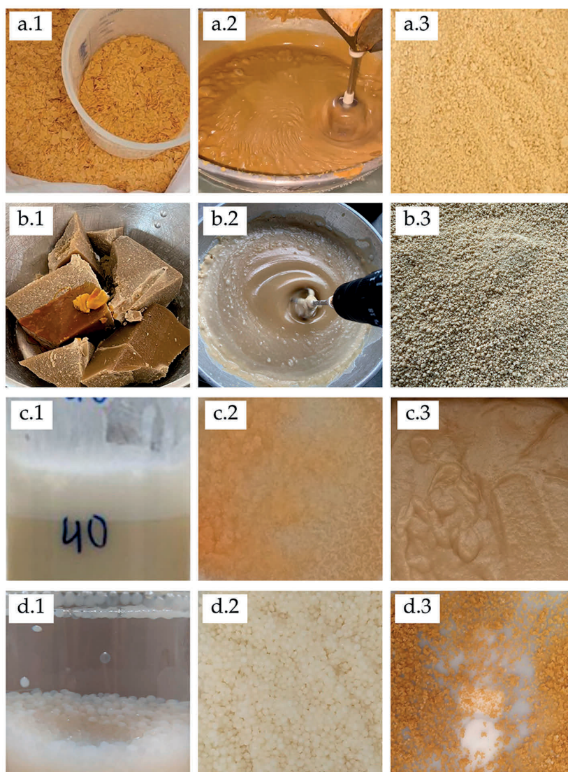
Figure 3. Different urea encapsulation systems using distinct wall materials. (a) [53,63] Carnauba wax: (a.1) pure wax flakes; (a.2) emulsion obtained by melting carnauba wax with urea and lecithin; (a.3) dried and ground material, showing a flour-like structure. (b) [52] Beeswax: (b.1) pure wax blocks; (b.2) emulsion obtained by melting beeswax with urea and lecithin; (b.3) dried and ground material, showing a flour-like structure. (c) [71,72] Vegetable fat: (c.1) emulsion prepared with vegetable fat, aqueous urea solution, and lecithin; (c.2) material after drying; (c.3) homogenized material with a pasty appearance. (d) [70] Sodium alginate: (d.1) beads formed by mixing urea with sodium alginate and immersing in calcium solution; (d.2) capsules after the gelification process; (d.3) dried material, showing a circular and solid structure. (Source: Photos by the author).
