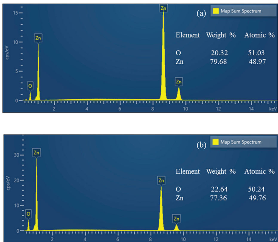
Figure 2. EDS spectra of hydrothermal (a) and sol-gel (b) ZnO.
