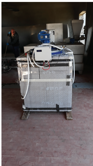
Figure 14. Prototype of a sludge mixing tank. Sludge, once sonicated, is deposited in a conveyor belt and fed into the prototype. Equipped with a temperature sensor and a humidity sensor, the prototype mixing tank heats the already ultrasonically treated sludge, further reducing the amount of water and consequently making it lighter.
