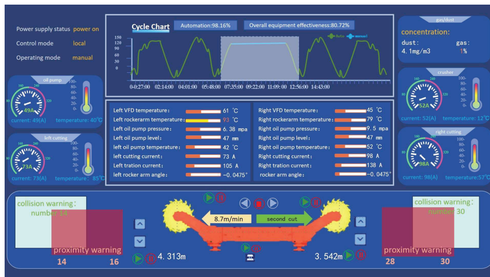
Figure 2. Example of shearer monitoring simulation task interface.
