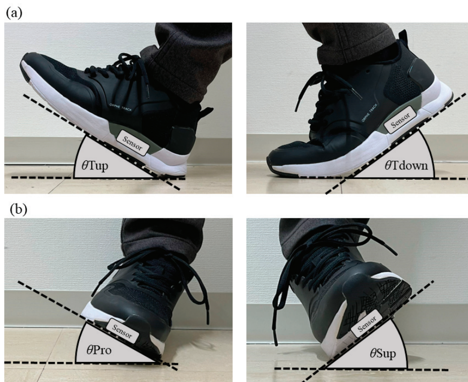
Figure 2. Parameters of shoe-floor angle. These parameters demonstrate the angle between the ground and shoe in the sagittal (a) or frontal plane (b) that were calculated through the sensor's anteroposterior or mediolateral axis and its projection vector to the horizontal plane. The angle of toe-up ( \theta_{Tup} ) and toe-down ( \theta_{Tdown} ) in the sagittal plane, and the angle of supination ( \theta_{Sup} ) and pronation ( \theta_{Pro} ) in the frontal plane were demonstrated.
