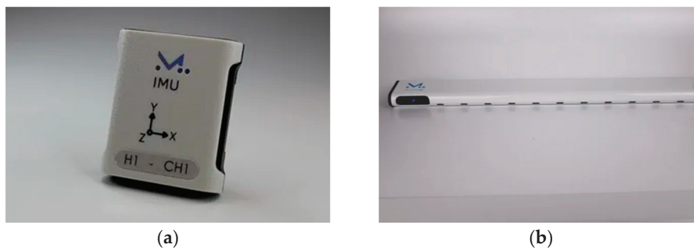
Figure 1. Inertial measurement unit (a) and contact grid (b) made by the Norwegian company MuscleLab https://www.musclelabsystem.com/products/ (accessed on 1 October 2025).
