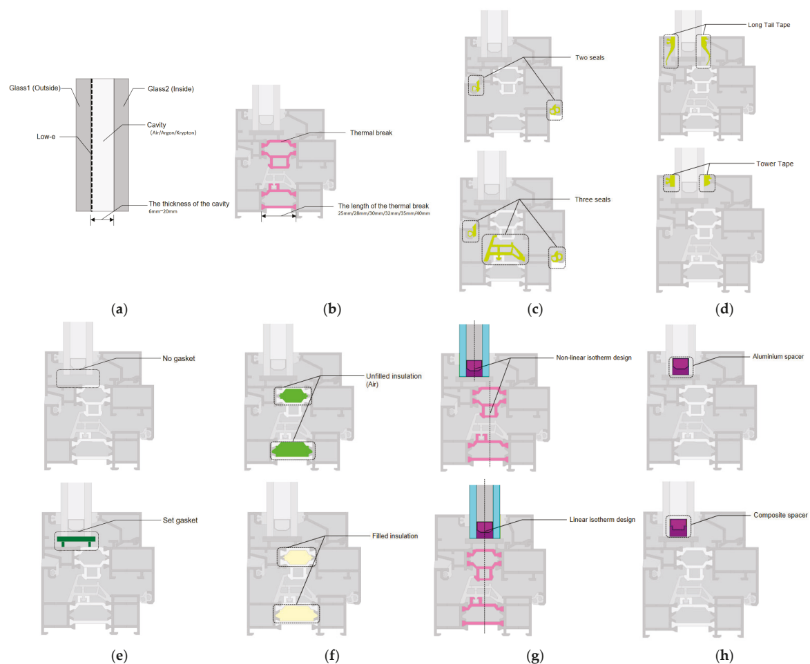
Figure 3. Graphical representation of the potential influencing factors on the thermal performance of broken-bridge aluminum exterior windows. (a) Double glazing; (b) thermal break; (c) number of sealing channels between the window frame and window sash; (d) the shape of the sealing tape; (e) whether or not to set the gasket under the glass; (f) whether the cavity is filled with insulation material; (g) isothermal design; (h) spacer types.
