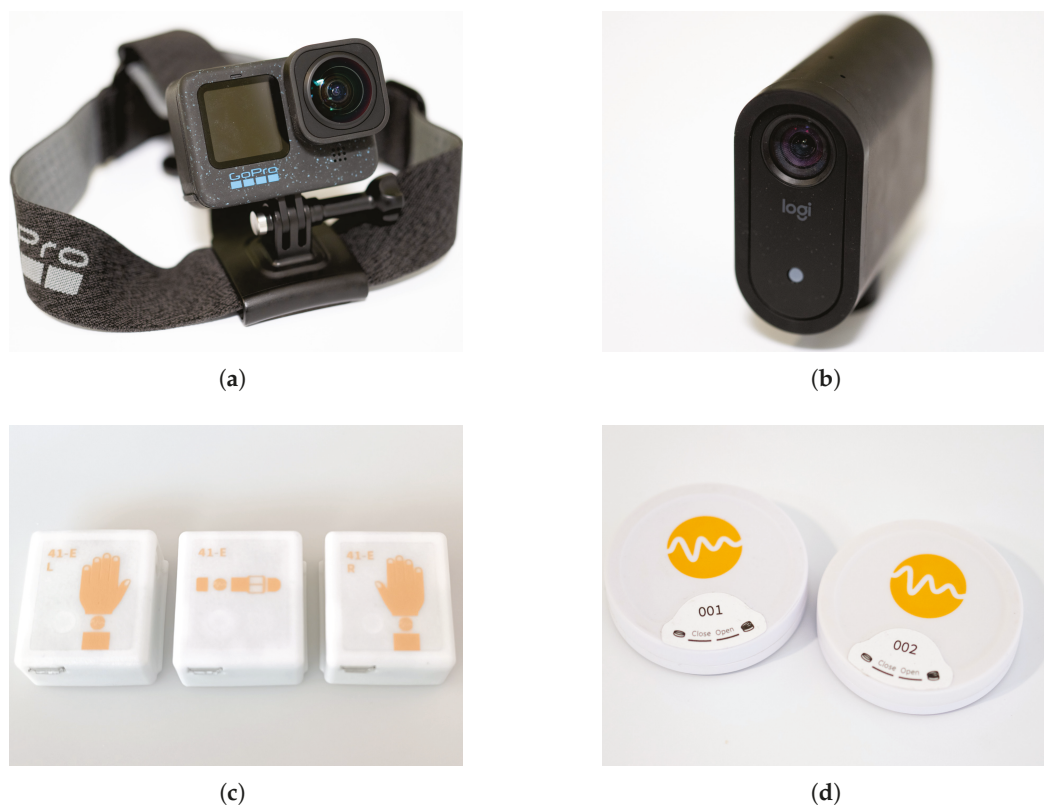
Figure 7. Sensors used to capture movements of the subjects and picking carts: (a) GoPro 12 action camera with ultra-wide-angle digital lens and head strap, (b) Mevo camera from Logitech without tripod, (c) one wearable set from MotionMiners with IMU and BLE sensors in each of the three devices, (d) first two beacons from MotionMiners.
