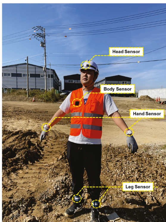
Figure 7. IMU sensor placement by body part.
