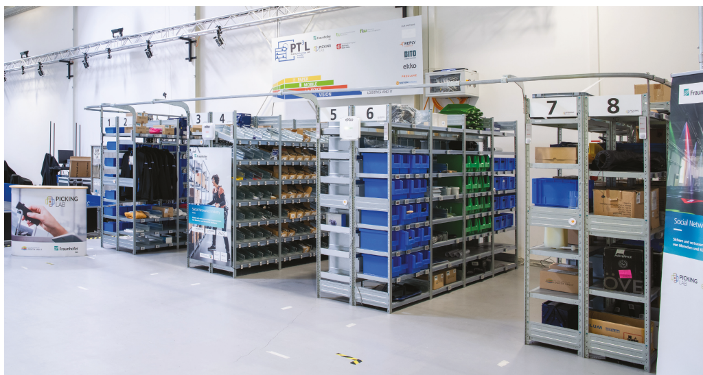
Figure 2. Picking Lab at the Fraunhofer Institute for Material Flow and Logistics (IML) in Dortmund, Germany. The photo shows eight numbered industrial rack complexes. The rack complex 1 stores small items in open-fronted storage bins. Complexes 2 and 3 hold hanging goods and loose items without bins. Complex 4 features flow channels for unboxed items and those in cardboard boxes. Complex 5 contains medium-sized flat goods, while complex 6 mainly stores medium-sized to bulky flat goods in green and blue open-fronted storage bins. Bulky and heavy items are located primarily in complexes 7 and 8.
