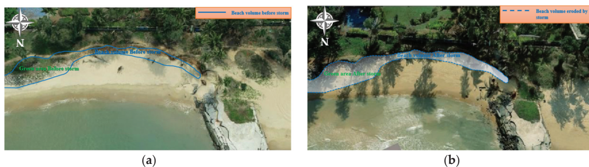
Figure 10. Beach berm with trees before (a) and after storm (b) in 2020 in Haikou Bay shows minor damage due to “green method” by storm waves.
