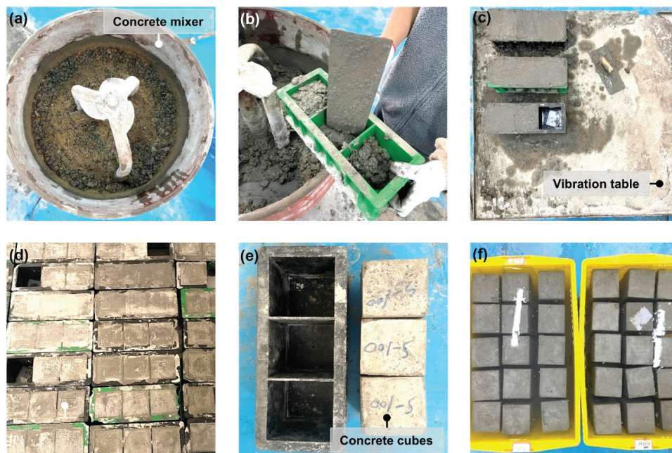
Figure 2. Preparation of the concrete specimen. (a) Stirring, (b) pounding, (c) vibration, (d) standing, (e) demolding, and (f) curing.
