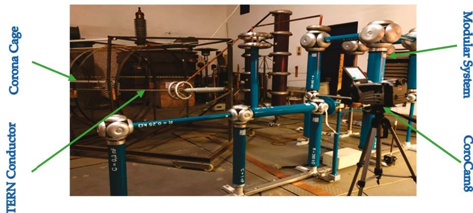
Figure 8. Test setup photograph with corocam8.
