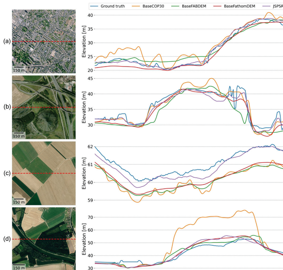
Figure 11. Elevation profiles by land use mask classes. The red-dashed lines are elevation cross-section projections on the remote sensing images. (a) Class 1 (urban fabric). (b) Class 2 (industrial, commercial, public, military, private, and transport units). (c) Class 5 (arable land (annual crops)). (d) Class 10 (forests) and 14 (water). (30 m to 3 m SR task, image + land use mask guidance).
