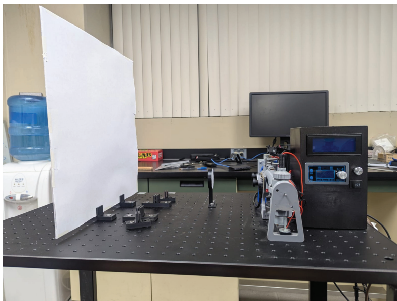
Figure 7. Experimental configuration showing the Technical Vision System (TVS), the stereovision module, and the planar calibration surface mounted on an optical breadboard.
