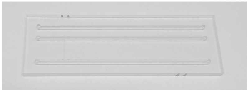
Figure 2. Example of a glass transfer standard chip, Design 04.
